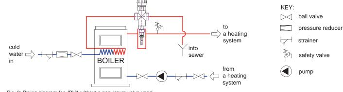
Pic. 3: Piping diagram for JBV1 without a non-return valve used
